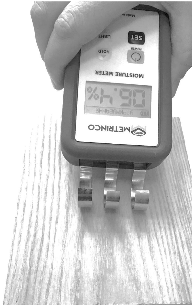
Figure 5 – Correct placement of the device sensor on a wood sample
